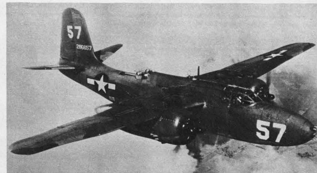
A-20G Flat Martin turret just behind the cabin is the recognitional change on the new Havocs. Engine changes have taken series to K, G and H have the solid nose, while the J and K have Plexiglass bomber noses and may carry three package guns on each side.
